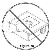
Lift the Top plate straight up to remove.
