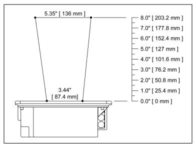
Figure 17: Scan Volume in Plane Perpendicular to Flow
