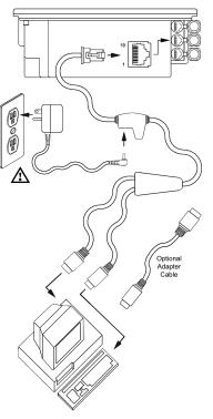
Figure 5: Keyboard Wedge Interfaces
