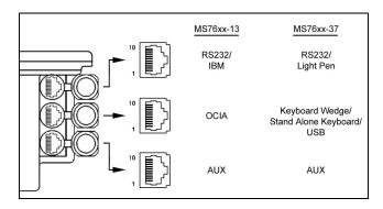
Figure 10: Connector Orientation (Top) Auxiliary Scanner Setup (Bottom)
