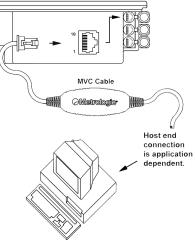
Figure 9: RS232/IBM, Interface
