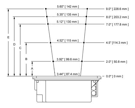
Figure 19: Depth of Field Perpendicular to Flow
