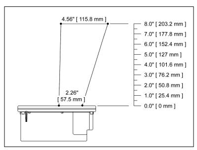
Figure 18: Scan Volume in Plane Parallel to Flow
