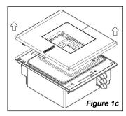
DO NOT PRESS on the window in the replacement Top plate.
