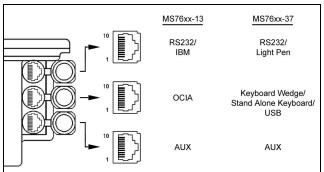
Figure 20: Scanner Interface Ports
