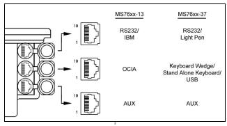
Figure 21: Scanner Interface Ports
