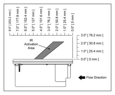
Figure 16: IR Activation Area Perpendicular to Package Flow
